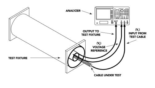
Shielding Effectiveness (dB)=  $20 \log (V_1) \frac{V_2}{V_2}$
