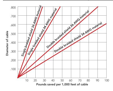
Weight savings realized by using Vermalloy® 3948 or ribbon copper shielding materials versus round shielding materials
